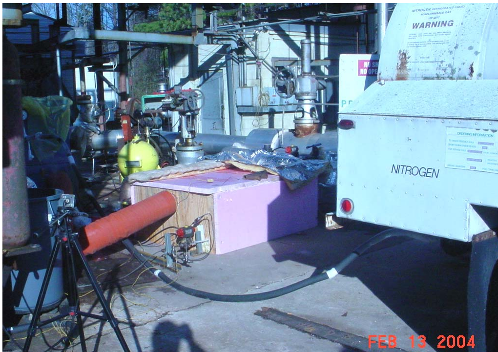
Photograph No. 10. Low Temperature Condition Setup
