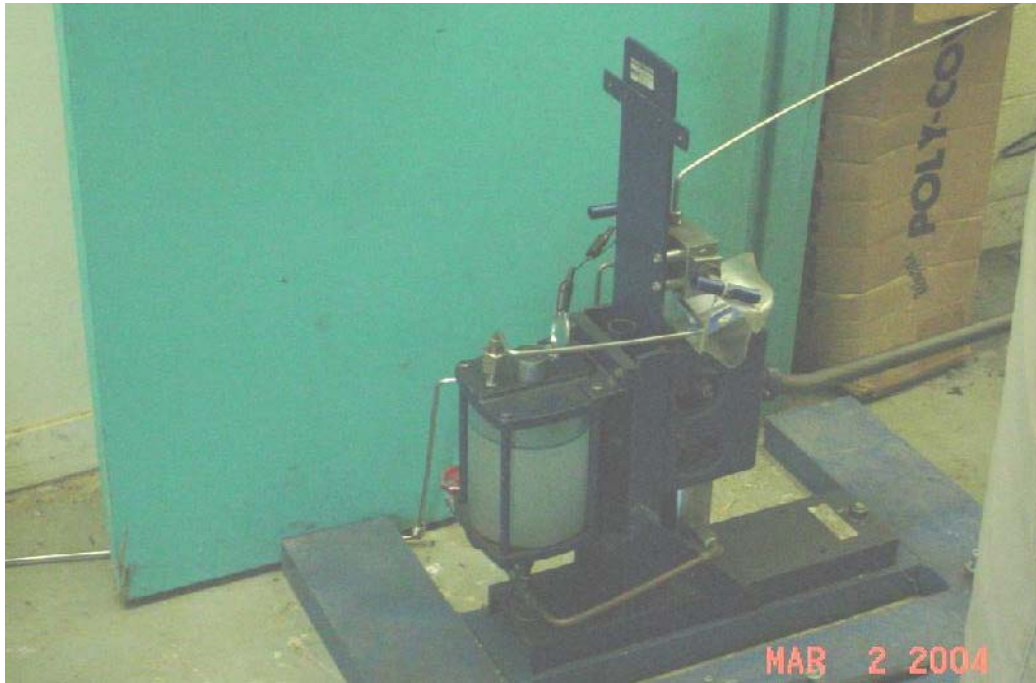
Photograph No. 17. High-Pressure Pump for Burst Test
