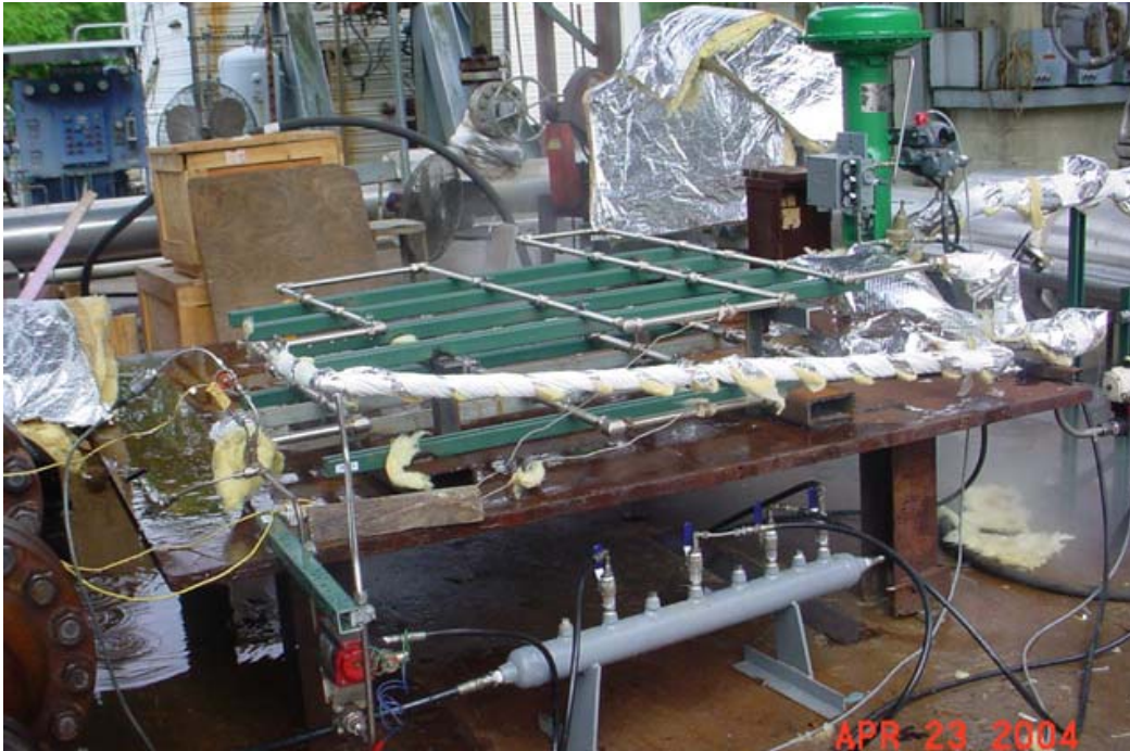
Photograph No. 9. Typical Setup for Temperature Cycle Testing
