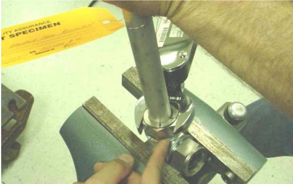
Photograph No. 1. Typical Torque and Assembly Technique
