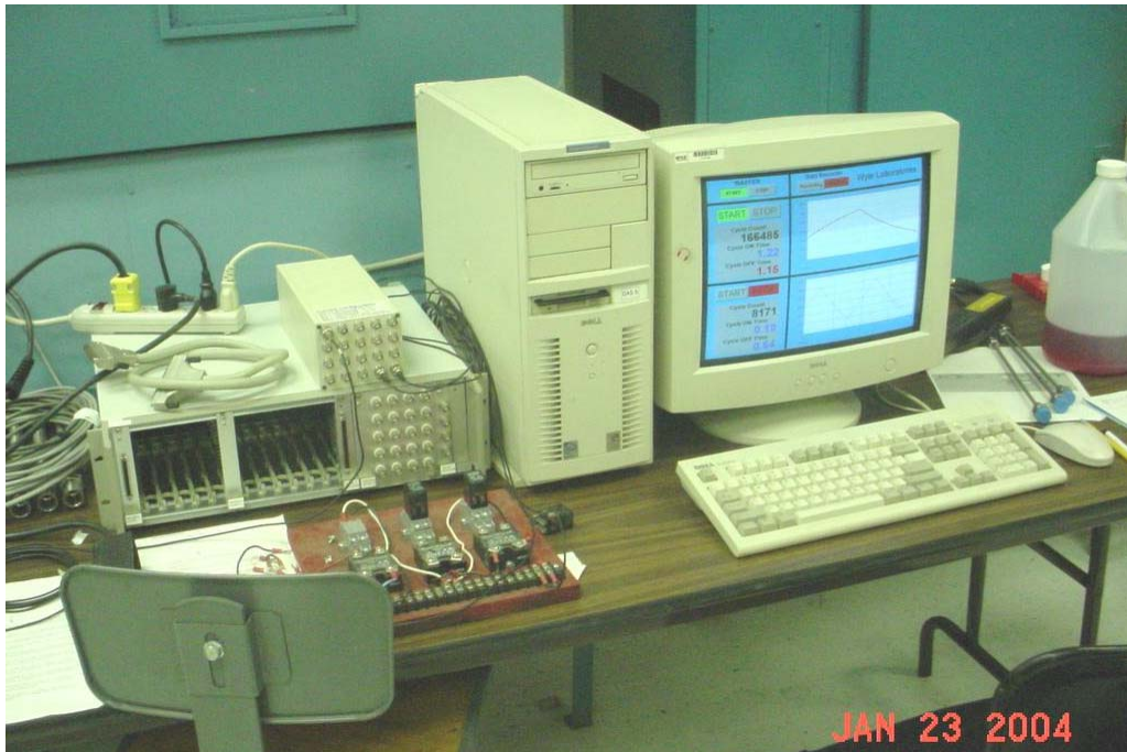
Photograph No. 12. Hydraulic Impulse Control System
