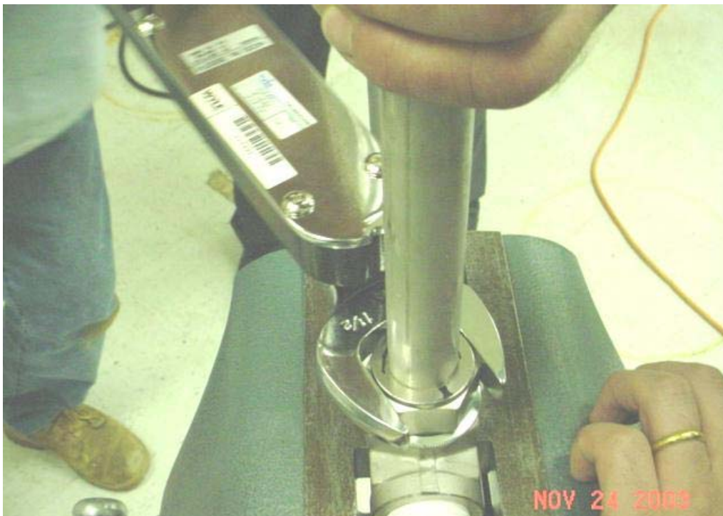
Photograph No. 2. Index Marking for Turn Identification
