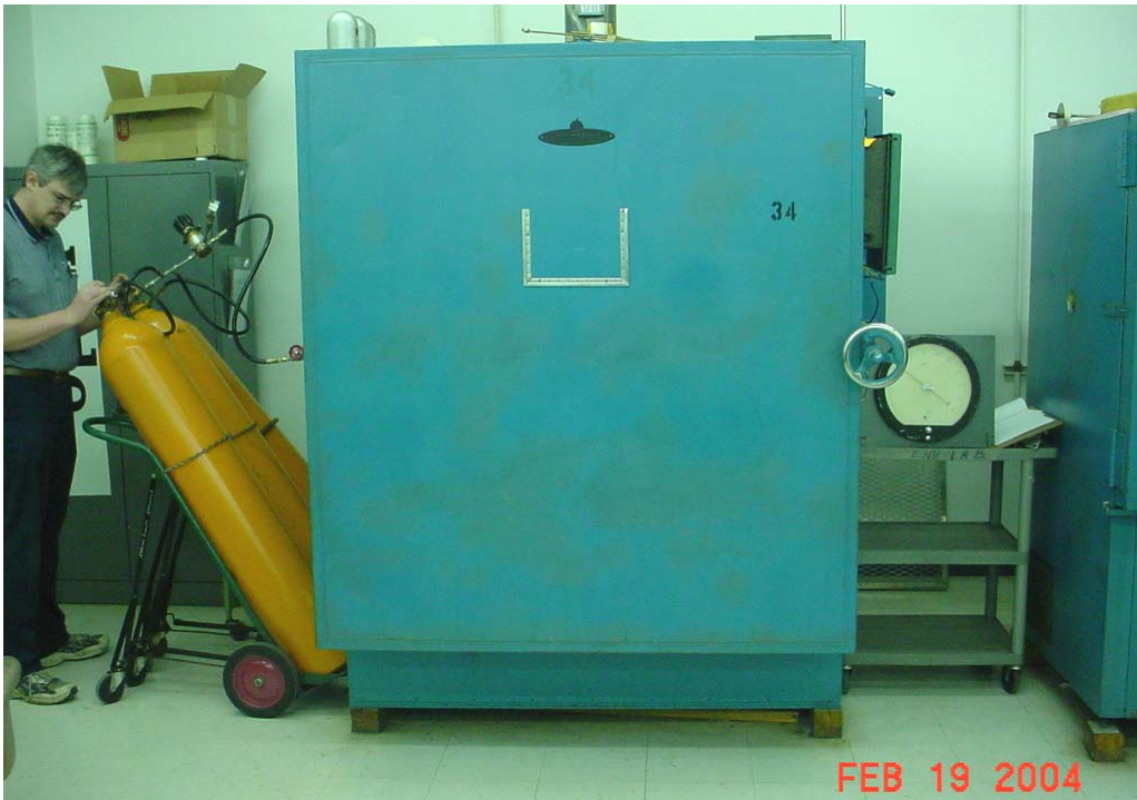
Photograph No. 14. Test Chamber for Elevated Temperature Test
