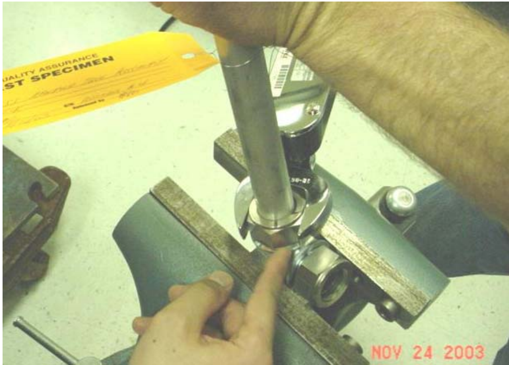
Photograph No. 3. Verifying Stop Collar Tightness
